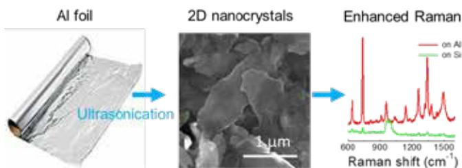
**Figure 1** Synthesis of Al 2D nanocrystals which show enhanced Raman scattering of adenine.
