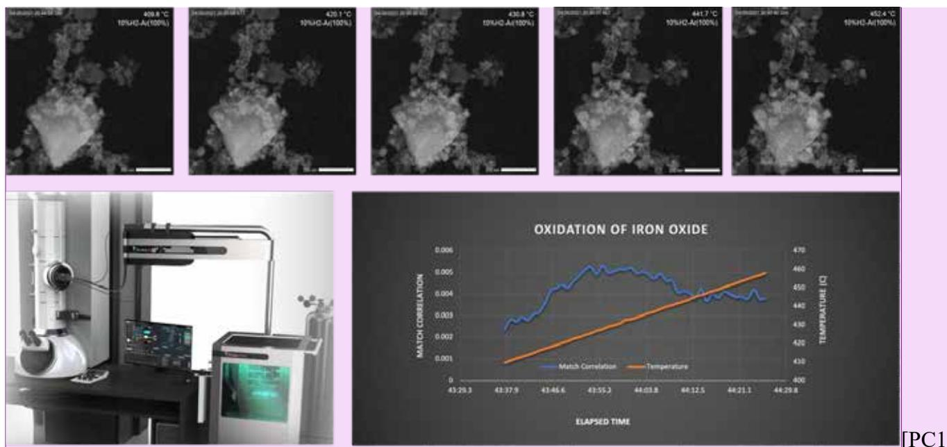
**Figure 1:** Reduction of Iron Oxide Nanoparticles Using a Commercial In-Situ Gas TEM System. Top Row: STEM images showing the morphological change in iron oxide nanoparticles during a heating ramp from 409°C to 452°C under a 10% hydrogen atmosphere. Bottom Left: Setup of the Protochips Atmosphere in-situ system on a TEM. Bottom Right: Metadata analysis using Protochips' AXON software.
