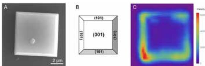
**Figure 1:** SEM image and Raman map of an anatase TiO<sub>2</sub> micro-crystal. A) Top view SEM image; B) Schematic diagram of anatase micro-crystal; C) Raman map of anatase E<sub>g</sub> mode at 144 cm<sup>-1</sup>.
