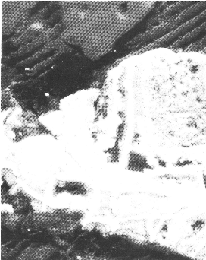
BACKSCATTER electron image of sample showing element differences more clearly than the secondary electron micrograph (above). The backscatter electron image is atomic-number dependent.
