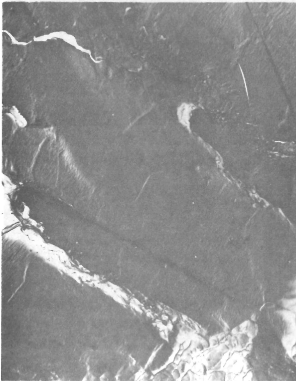
Figure 6. Fractographs from selected locations in fracture surface of laboratory fatigue test specimens. 3000X
