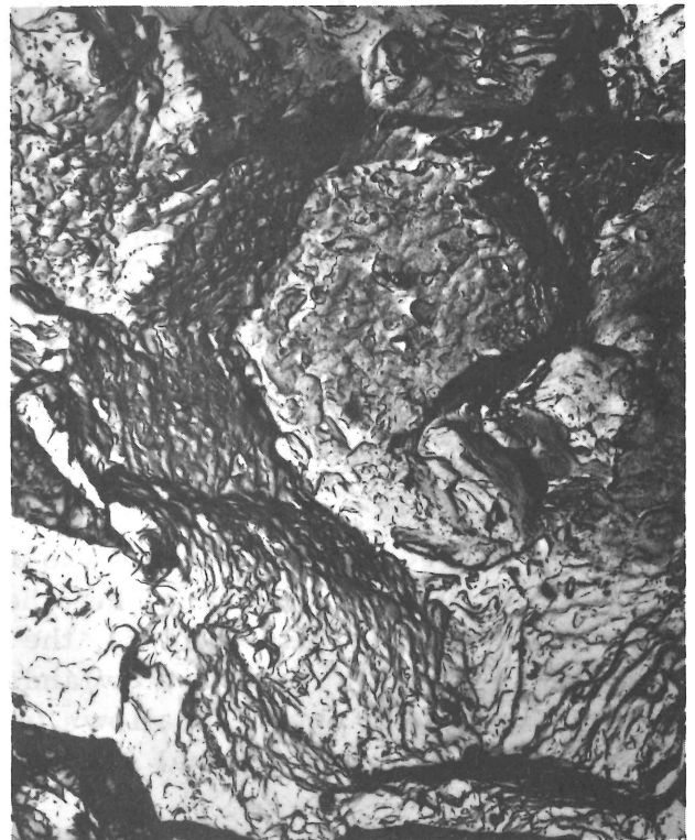
(b) Abnormal material. Predominance of intergranular fracture. 2000X
