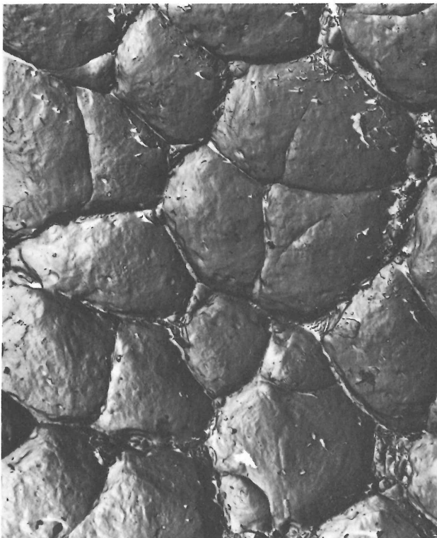
Figure 3. Transgranular portion of fracture surface of overaged Al-4.2% Cu notched-tensile specimen. 2000X
