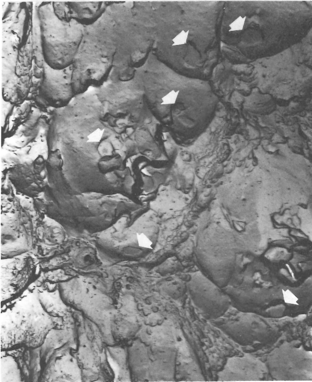
Figure 1. Fractograph from notched-tensile specimen of 2017 aluminum alloy aged 10 hrs at 450°F. Arrows indicate void initiation sites. 2000X
