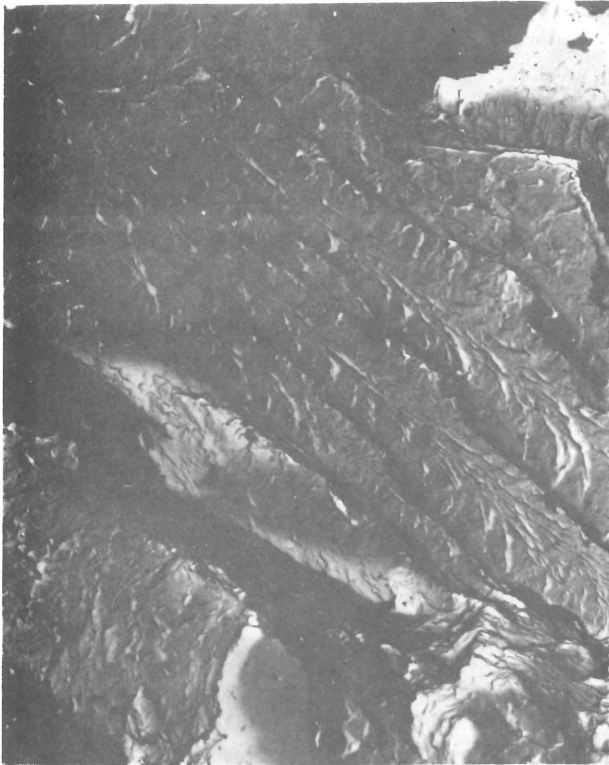
Figure 5. Examples of "step-type" topography of service-induced cracking in forged aluminum compressor discs.
