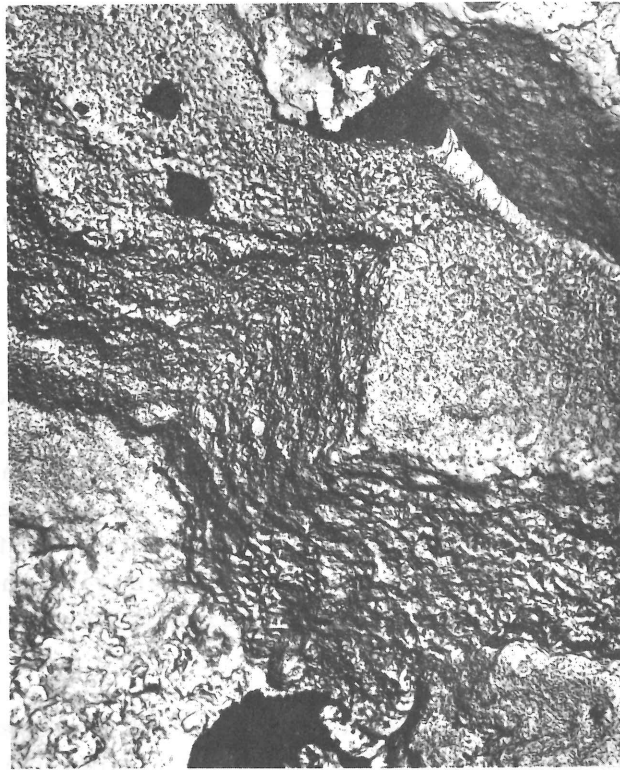
Figure 7. Fractograph from fracture initiation zone of A-437 pressure vessel closure stud. 2000X
