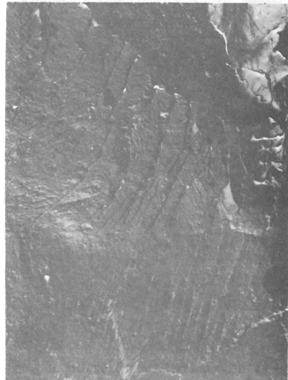
Figure 6. Fractographs from selected locations in fracture surface of laboratory fatigue test specimens. 3000X
