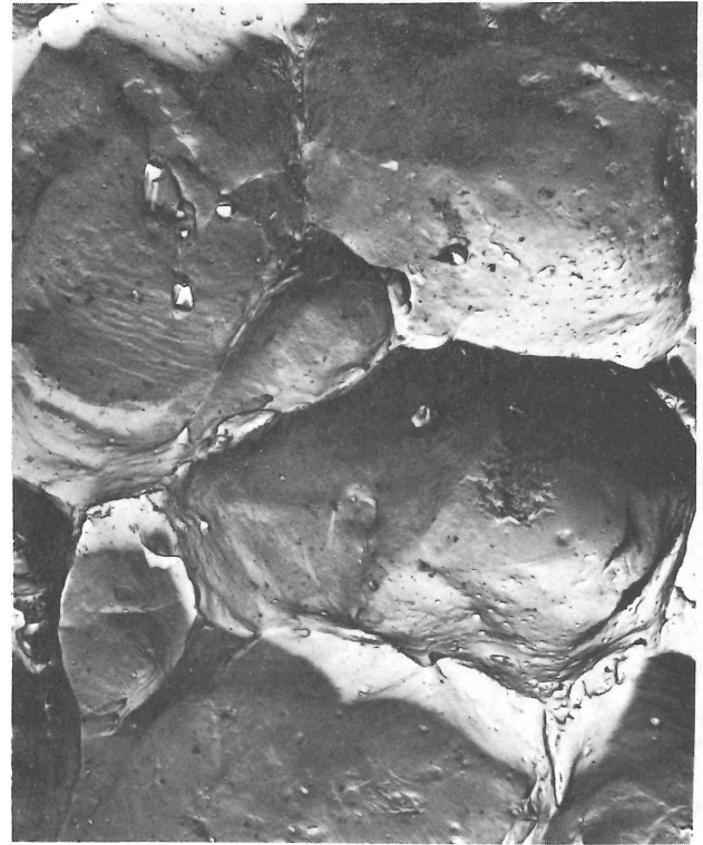
Figure 2. Large uniform dimples in fracture surface of a 6061 aluminum alloy notched-tensile specimen. 2000X
